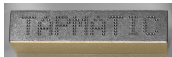
Point to point programming for creating characters with defined dot position or 2D Data Matrix codes.
